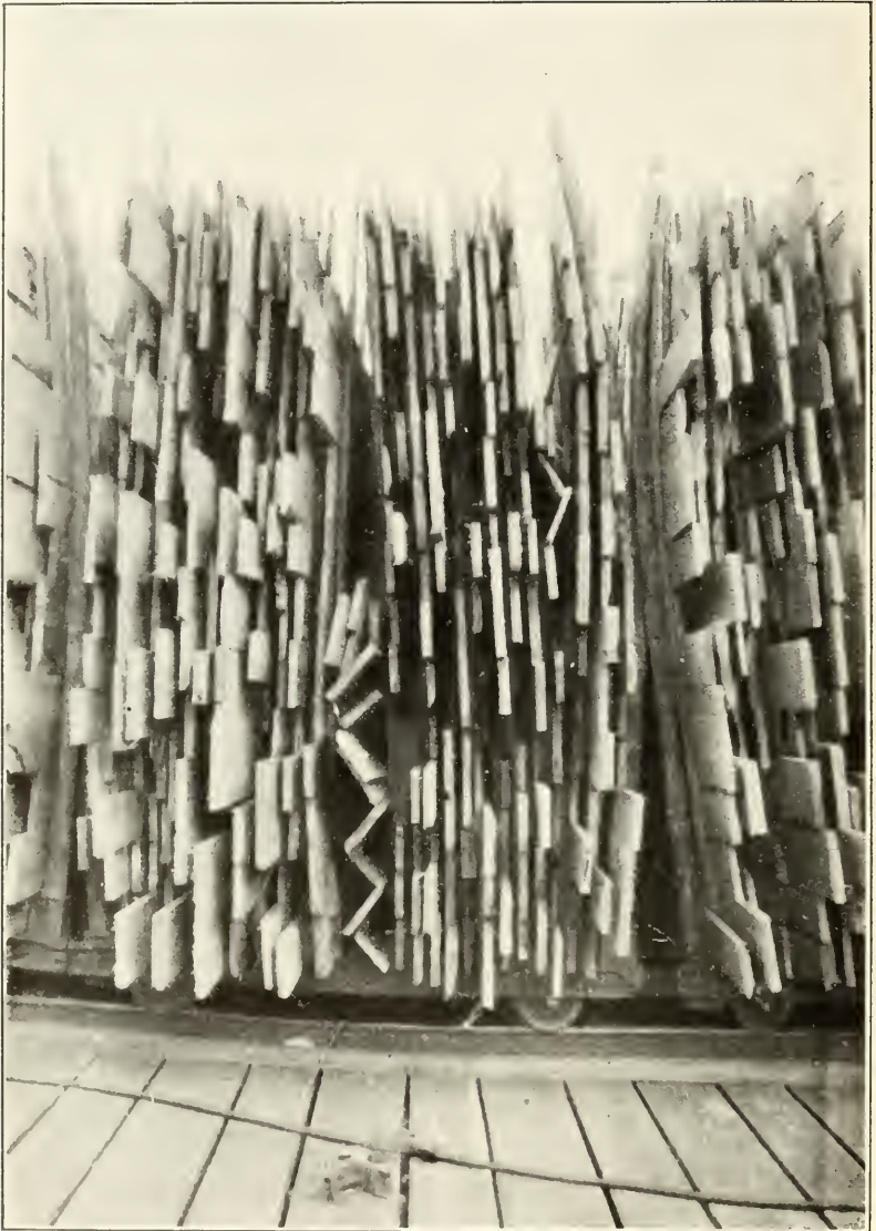
Edge-stacked lumber with tumbled tiers as a result of carelessness at the time of stacking. The position of the lumber causes poor drying in such tiers and often causes severe checking also. Shrinkage during drying sometimes results in tumbling as bad as this, especially when automatic take-up devices are not used or are inadequate
